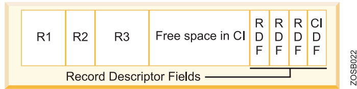
Figure 12. Simple VSAM control interval
